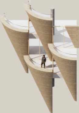
The prefabricated shells can be rapidly lifted upon a concrete framework.
